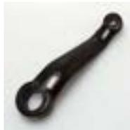
Note: This arm is slightly longer than factory, measuring 6-7/32" center to center.
