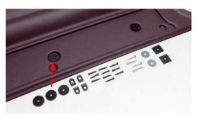
**Step 6:** Prior to installing the screws on the bottom portion that fit beneath the carpet insert panel, make sure to install a scotch-lock on each screw. This scotch-lock will be used to hold the carpet insert panel in place (you will see corresponding scotch-locks on the back of the insert panels).
