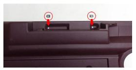
**Step 4:** Start the installation by attaching the door panel with the factory screws located on the top edge behind the arm rest. Use the supplied D-shaped washers on each screw. These washers will help strengthen this area of the panels since much of the force of closing the door happens here.
