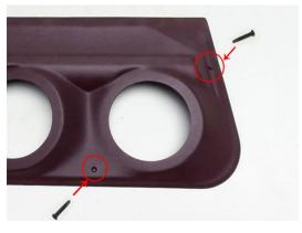
**Step 5:** With the 2 upper screws loosely tightened in place, you can now locate the screw holes along the bottom and front edge. Once you have the panel level with your door shell and upper door panel, attach the screws in front of and below the speaker pods. Each screw is self-tapping so there is no need to pre-drill the holes unless you prefer to.
