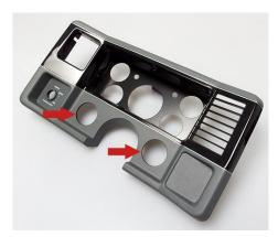
**Step 4:** Once mounting holes are drilled, the shadow box is ready for final install. If you require a couple more gauges than the shadow box allows, use a 2-1/16" hole saw to drill (2) holes on either side of the steering column as shown here.
