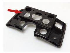
**Step 2:** It fits over the back of the factory faceplate. Once in place, mark the mounting holes and remove the shadow box from the faceplate.
