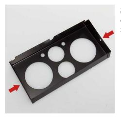
**Step 1:** Your new shadow box allows aftermarket gauges to be mounted directly to the gauge faceplate. The box mounts with 2 bolts on the left and right side of the faceplate.
