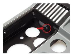
**Step 3:** Once you have marked the hole locations, drill your holes to the appropriate size. We like to use M5-1x10mm black button head bolts/nuts but you can use any hardware up to  $\frac{1}{4}$ ? diameter.
